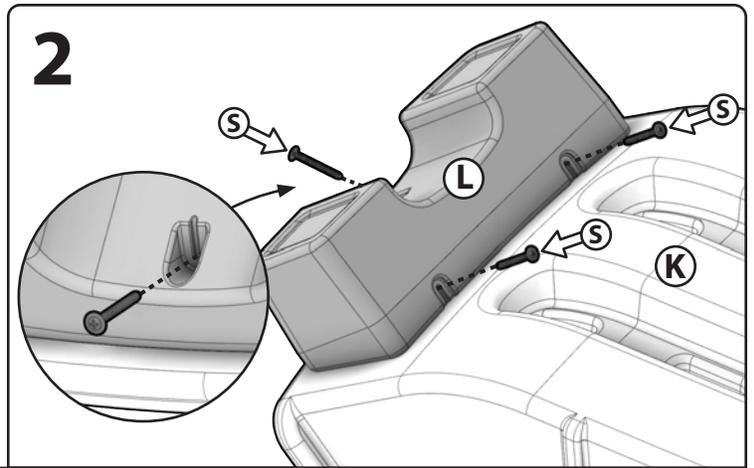
**STOP!** Double check that correct screws are used.
