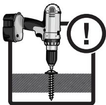
**DRILL TIPS:** Product has no holes. Screws form their own. Adjust drill torque to lowest settings. Increase incrementally to drive screw head flush with surface. DO NOT OVER TIGHTEN.
